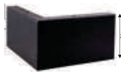
W07 Plywood, painted black
